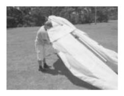
13. Attach the sail ties loosely around glider, going from the wing tip to nose. Then tighten the ties, moving from nose to wing tip. Adjust the sail such that the leading edge Mylar inserts overlap smoothly with no kinks, as shown.
