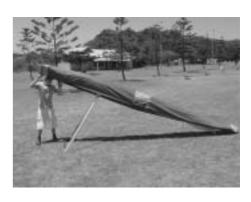
15. Disassemble the control frame. Fold the base tube out and lay the entire control frame assembly back onto the keel. Open the ties and re-secure them over the control frame, enclosing the frame with the leading edge pockets. Fit the padding provided to the bottom of the control frame. Tuck all wires and bars neatly inside the sail. Pull the hang loop from in front of the uprights so as not to jam the hang loop between the keel and sail.
