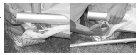
Repeat 1-4 to install the left back section. Your Litesport will now be ready for standard assembly. Before each flight, carefully inspect all tubing, nuts, and bolts, to ensure no damage has occurred during transportation.
