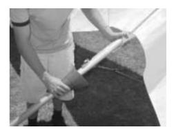
12. Fold and roll the sail parallel to the transversal battens.
